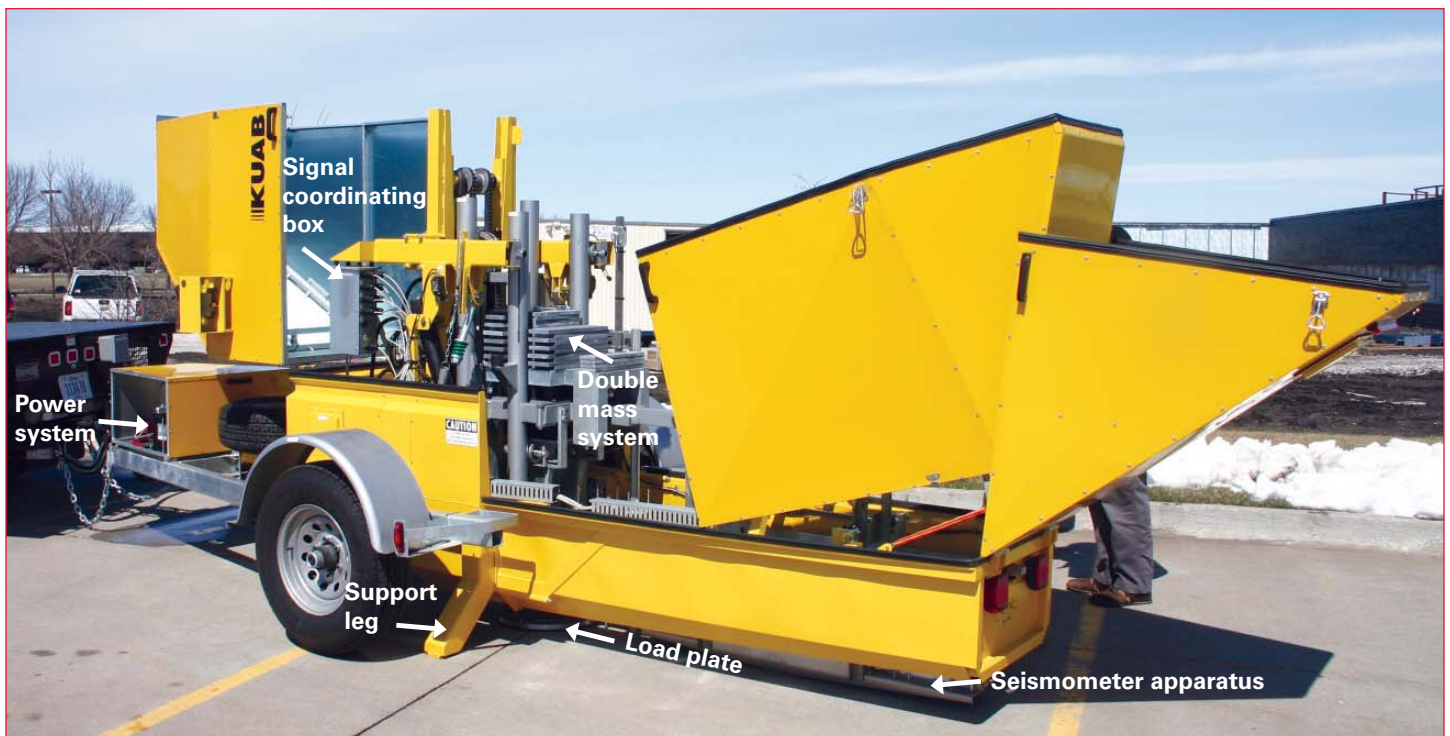
Loading system hoisted on support legs in testing position, seismometers and load plate resting on the surface, protective shell open
