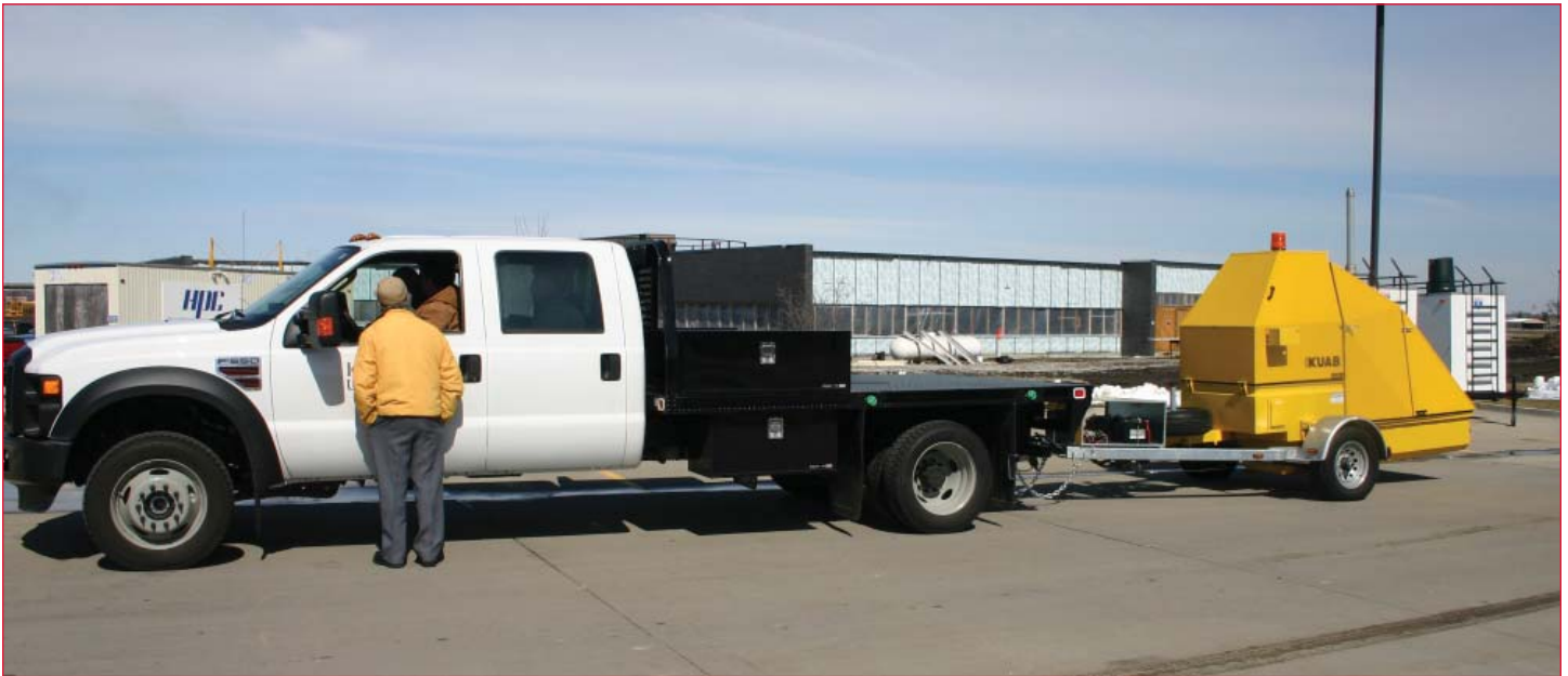
KUAB Model 150 2m falling weight deflectometer pulled by towing vehicle
